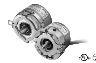
The optical Sendix 5873 singleturn encoders with SSI or BiSS interface and optional 2048 ppr SinCos incremental track reach a resolution of up to 21 bits.
